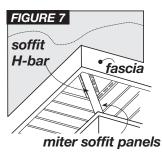
If necessary, install nailing strips to provide backing for the lineal. Cut and install soffit double channel lineal or H-bar (see figure 7). Miter the corner soffit panels and install as described above.
