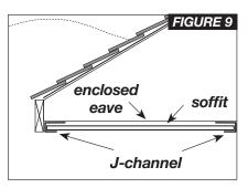
The procedure used to install soffit over an enclosed eave is almost identical to that used for an open eave. The major difference is the installation of the J-channel. Determine the method you'll use to install soffit at the fascia board (see figures 8 and 9). When installing J-channel at either the wall or the fascia board, nail the J-Channel every 12"-16".
