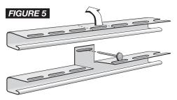
wall. After cutting the nail flange, bend the flange back and nail to the wall. When installing Beaded T2" panels, use 3/8" H-bar or 3/8" J-channel.
