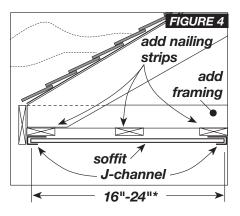
If no F-channel is available, J-channel can be modified to create F-channel. Simply cut slots (as shown in figure 5) in the nail flange area where it would be nailed to the
