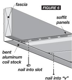
If you're using a nailing strip (as in figure 4), do not nail tightly—allow movement for expansion.
